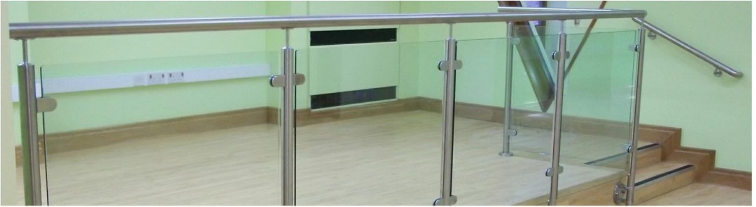
Steelcraft offers balustrade and matching handrail in internal-grade 304 or external-grade 316 stainless steel available with either satin or mirror-polished finishes.
